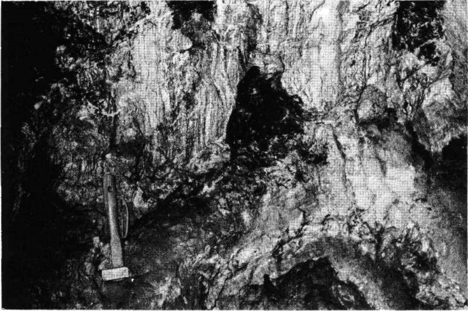
Fig. 2: Face of underground-working into stratiform ore-rich illitic layers (Rotenstein near Serfaus; exp. 1, area L).
