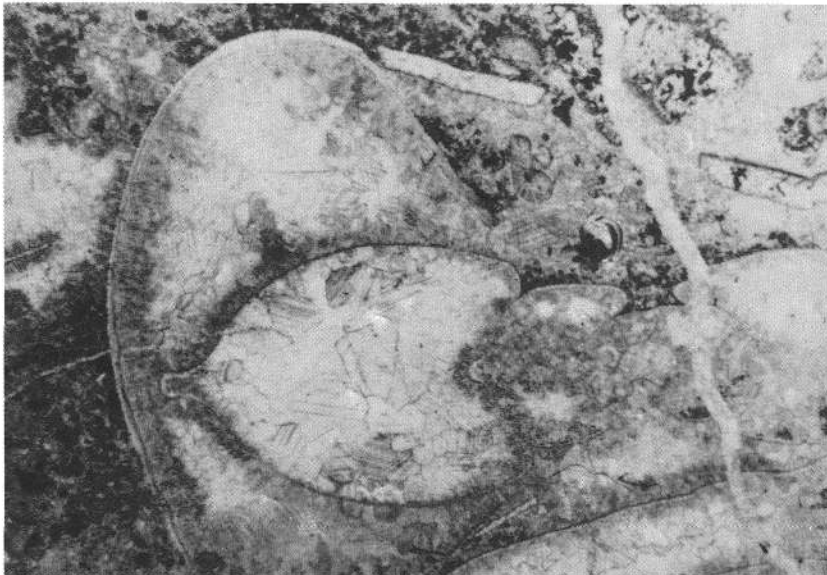
Fig. 9. Hierlatz limestone: biosparite, grainstone with small ammonite. The "isopachous" radial-fibrous sparite that precipitated during the first phase is well separated, due to its darker shade, from the later, mosaic-like sparite. Szentgál, Tűzköves-hegy; Sinemurian, ca. 8x.
