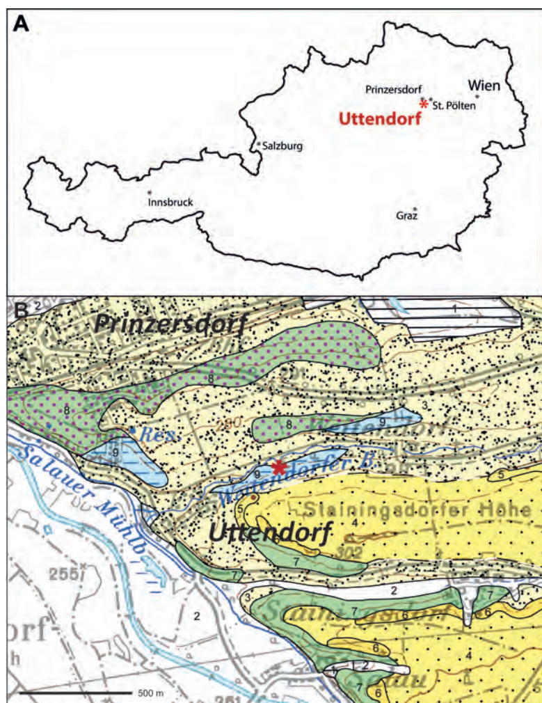
Text-Fig. 1. A. Location of outcrop within Austria. B. Geological map of surrounding of sample location southeast of Prinzersdorf (from map sheet 55 Ober-Grafendorf, SCHNABEL et al., 2012). Explanation of lithologic units: 1 Antropogenic cover, 2 stream and river deposits, 3 solifluction and sheetflow deposits, 4 Loess and Loess loam covering gravel terraces, 5 younger gravel terraces (“Jüngere Deckenschotter”), 6 older gravel terraces (“Ältere Deckenschotter”), 7 “ Robulus -marl” (lower Ottnangian), 8 Prinzersdorf Formation (lower Ottnangian), 9 “Älterer Schlier” (clay and marl, upper Egerian).
