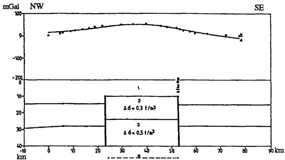
Fig. 1. Gravity model calculation along the seismic profile K-1 (for suddenly descending model)
