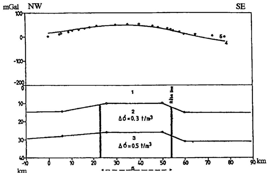
Fig. 2. Gravity model calculation along the seismic profile K-1 (for slowly descending model)
