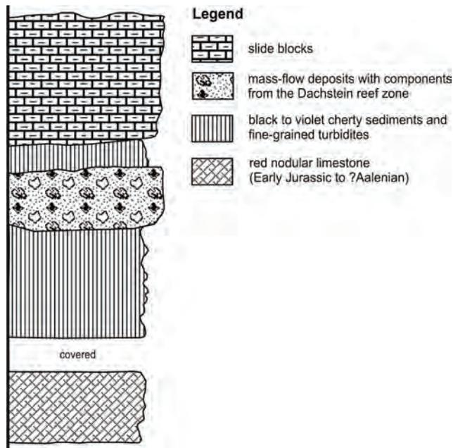
**Figure 28:** Generalized sedimentary succession of the Büchsenkopf area. The contact between the Early to Middle Jurassic red nodular limestones is not exposed. The black radiolarites below the first mass-flow deposits are dated as Callovian by means of radiolarians. The first resediments occurred in the Oxfordian according to GAWLICK et al. (2003) and MISSONI (2003). The thickness of the whole preserved succession does not exceed 150 metres. The section is not to scale.
