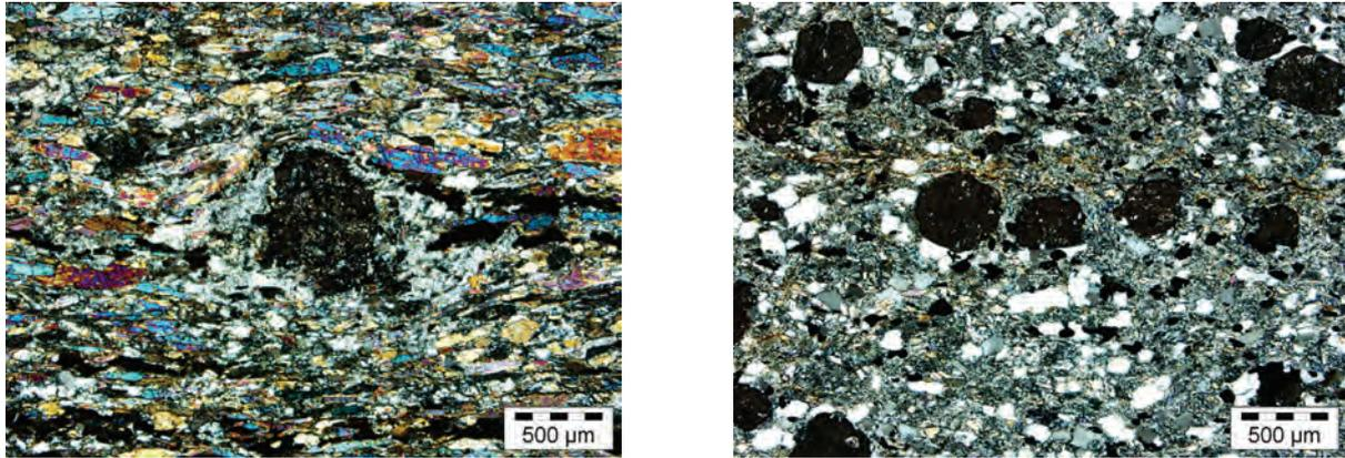
**Figure 9:** Microfabric and texture of retrogressed garnet amphibolite; garnets show rims of chlorite and epidote (left); retrogression of hornblende to fine-grained symplectite (right).
