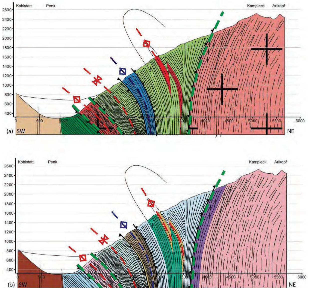
**Figure 22:** Profiles 3 (trace and legend in Figure 26) near Oberkolbnitz: (a) tectonic units, (b) lithology. D5 folds marked in red, axial traces of D3 (blue), D4 roof thrust of the Venediger Duplex (green).
