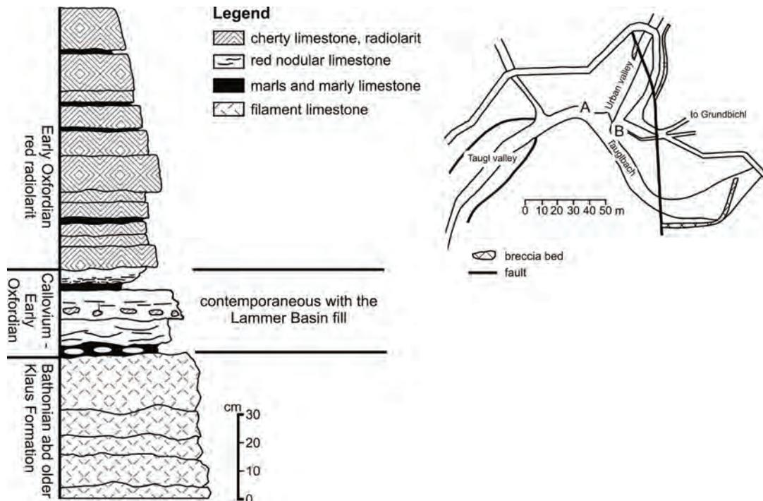
**Figure 30:** Area of the Urban creek/Taugl creek in the central Salzburg Calcareous Alps, exposing excellent sections of the succession around the boundary Klaus Formation/radiolarite (Tauglboden Formation) in the. The drawn detailed section is from west of the Urban valley (A). An equivalent section is seen east of the Urban creek (B). Redrawn after HUCKRIEDE (1971).
