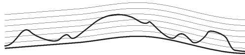
Fig. 1: Schematic depiction of INCA coordinate surfaces. The vertical coordinate is the height above the valley floor surface, which forms the base of the topography. Vertical resolution is 200 m.
