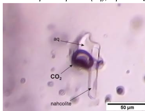
Fig. 2. Three phase fluid inclusion comprised of aqueous phase (aq), liquid \text{CO}_2 and nahcolite crystal
