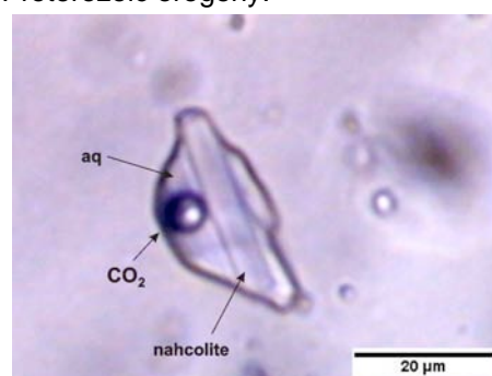
Fig. 1. Nahcolite crystal enclosed within inclusion comprised of aqueous phase (aq), liquid \text{CO}_2
