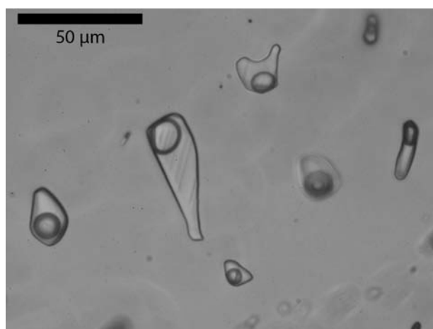
Fig. 4. Synthetic \text{H}_2\text{O}-\text{NaCl} fluid inclusions of variable sizes and shapes with an eutectic composition (23.3 mass% NaCl)
