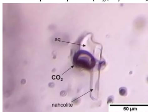
Fig. 2. Three phase fluid inclusion comprised of aqueous phase (aq), liquid  $\text{CO}_2$  and nahcolite crystal
