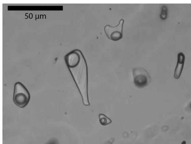
Fig. 4. Synthetic  $\text{H}_2\text{O}-\text{NaCl}$  fluid inclusions of variable sizes and shapes with an eutectic composition (23.3 mass% NaCl)
