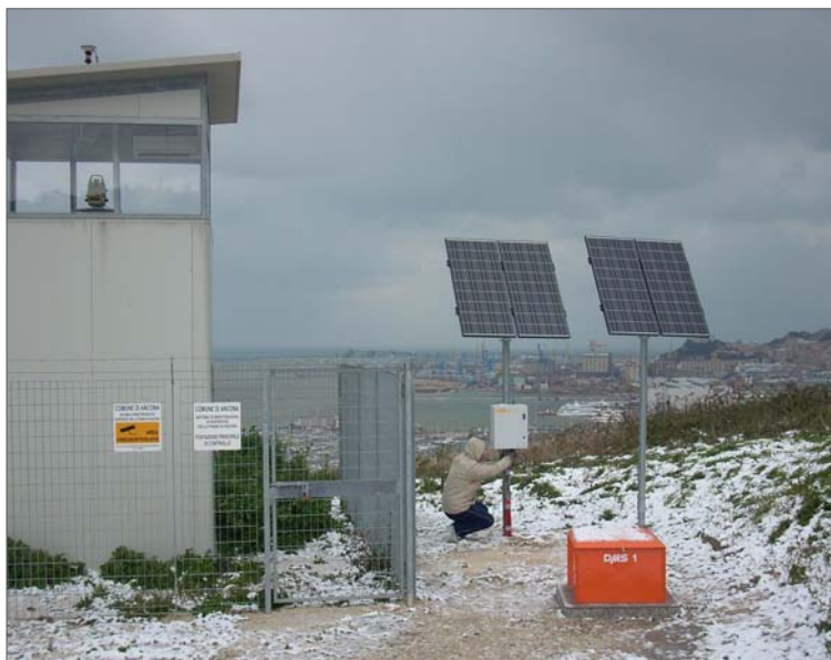
Fig. 4: Surface and geotechnical DMS-systems (Via delle Grotte site).
