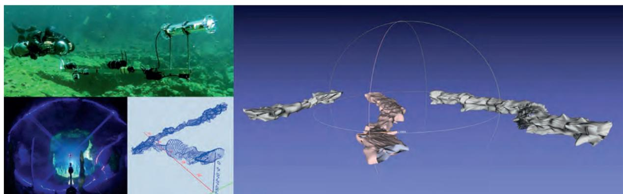
approximately 800 cross sections have been captured in six tunnels. With an average separation of two meters in mean this gives about 1,600 meters of scanned tunnels producing six 3D-models of karst conduits.
