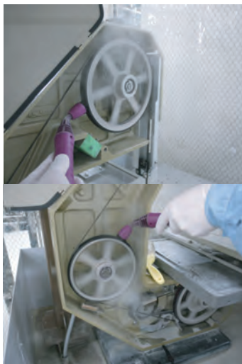
Figure 3. Cleaning run. Band saw and three wheels must first be cleaned with heat-steam followed by an ethanol spray-wash and a Milli-Q rinse.
