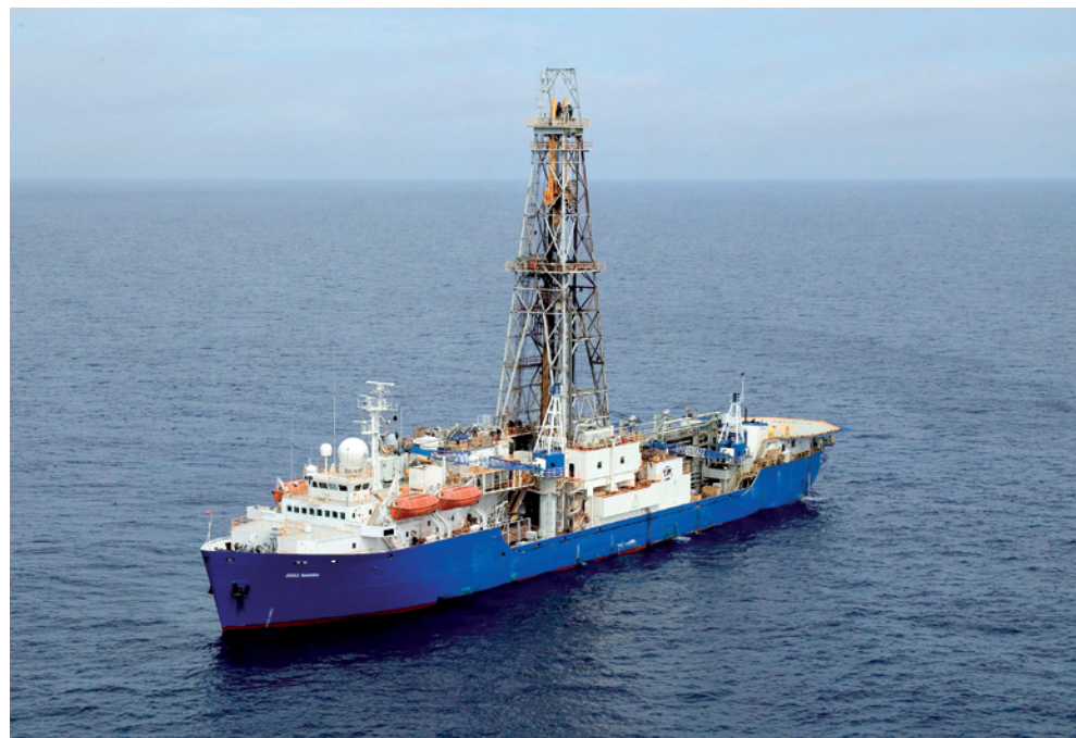
Figure 1. The pre-modernized JOIDES Resolution , an ~143-m-long, dynamically positioned drill ship, with a derrick extending >61 m above the water line, began operations in 1978 as the SEDCO/BP 471 and was converted in 1985 for use by the Ocean Drilling Program (ODP). The derrick height and overall size allow this vessel to be able to access a wide variety of ports, including passing under the Bridge of the Americas (Panama) and the Golden Gate Bridge (San Francisco, California). The name came from the JOIDES (Joint Oceanographic Institutions for Deep Earth Sampling) advisory structure and after the HMS Resolution , the vessel of exploration commanded by Captain James Cook. By the end of ODP and during initial IODP operations, the JOIDES Resolution (JR) included a fully equipped lab stack, the scientific heart of expeditions, equivalent in its fitting and capabilities to shore-based research laboratories.
