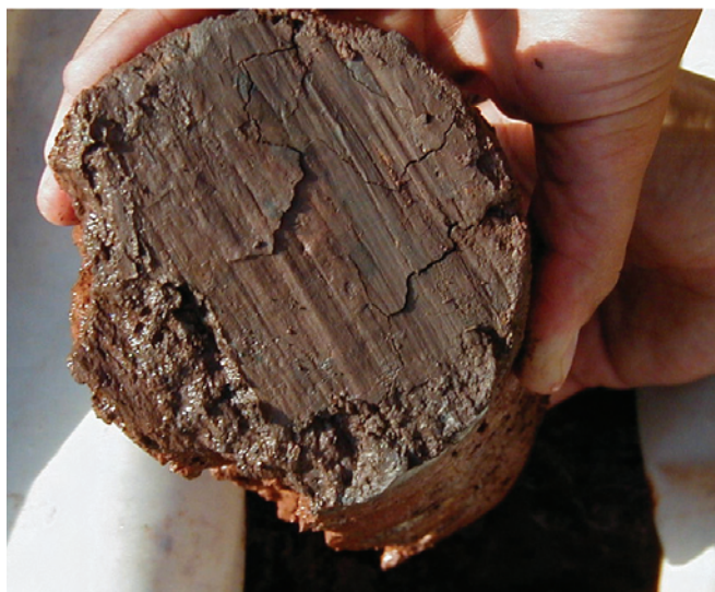
Figure 2. Slip lines observed on the slip surface of the Corinth core.
