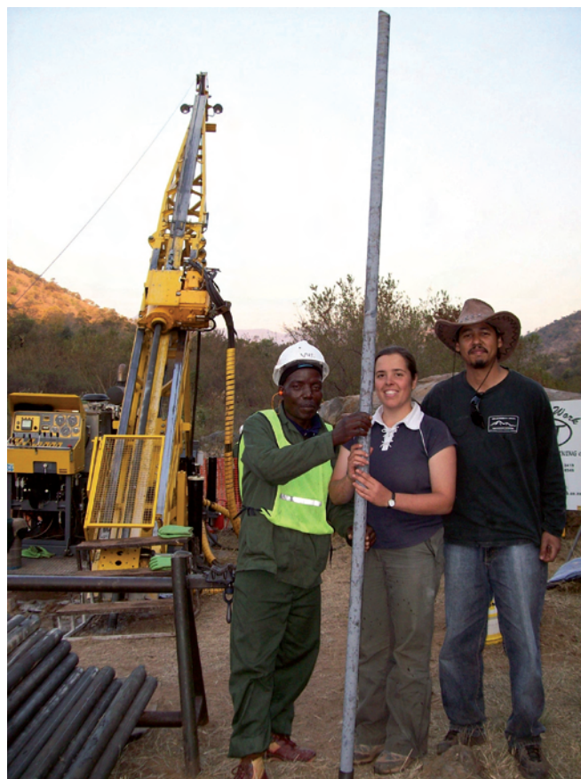
Figure 2. Drill rig aligned and set to drill at the shallowest possible angle ( 45^{\circ} ) relative to the dip and dip direction of the steep near-vertical orientation of the geological units along the Komati River. The >3-m-long rod is composed of basalt or diamictites.
