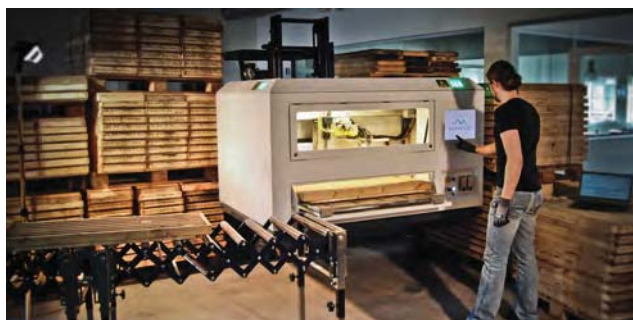
Figure 1. The new instrument described is a drill core scanner that intelligently handles entire drill core trays to produce chemical analyses of drill cores.
