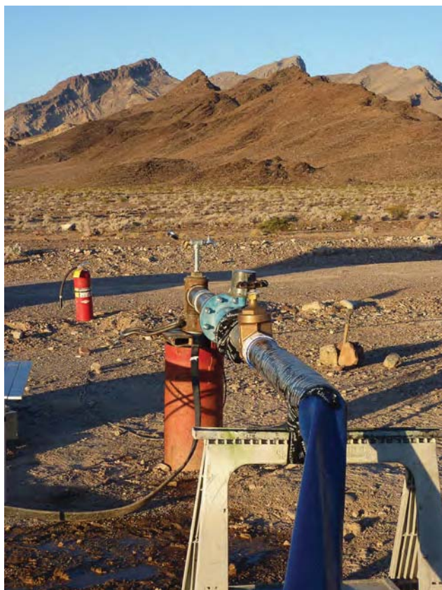
Figure 5. Possible drilling site near Death Valley, California, on the eastern flank of the Funeral Mountains. A consortium of interests, including the U.S. Department of Energy, U.S. Geological Survey, Inyo County, California, and the Hydrodynamics Group, LLC, drilled a well (BLM-1) to 883 m depth through a range of sedimentary and volcanic lithologies and conducted two hydrologic pump tests. The underlying carbonate aquifer contains anoxic thermal water (58 °C) and abundant sulfate-reducing bacteria including Candidatus Desulforudis sp. and Desulfotomaculum spp. (Thomas, 2013).
