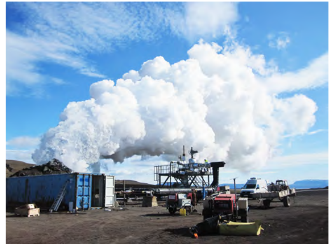
Figure 3. The flow of the IDDP-01 into a rock muffler produced dry superheated steam with only 0.1–0.2 % of non-condensable gases. Initially corrosion products gave the steam a dark color, but after a few minutes it became clear and transparent. The condensate had a pH of 2.5–3 due to its HCL content. However, experiments on wet scrubbing to remove acid gases from the dry steam were very successful (Hauksson et al., 2014) (photograph courtesy of Kristján Einarsson).
