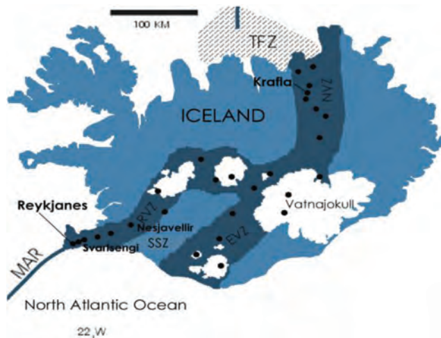
Figure 1. The slow spreading ( 2\text{ cm a}^{-1} ) Mid-Atlantic Ridge (MAR) connects with central neovolcanic rift systems of Iceland (dark blue). Black circles are high-temperature geothermal systems. RVZ = Reykjanes Volcanic Zone; EVZ = Eastern Volcanic Zone; NVZ = Northern Volcanic Zone. The SSZ = Southern Seismic Zone and TFZ = Tjorness Fracture Zone. The white areas are glaciers.
