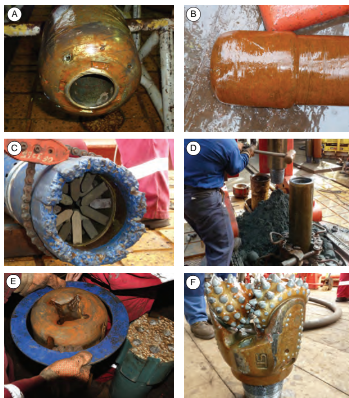
Figure 6. Photographs of some drilling, fishing, and milling tools illustrating the multiple operations achieved during IODP Expedition 335. [A] & [B] Remains of the Ultra C9 RCB coring bit used during Run 9. The bit was probably used for ~10 h after it disintegrated, which resulted in this spectacularly abraded and sculptured bit ("Stumpy"), something never seen before by the drillers. [C] Bottom of the Bowen Reverse Circulation Junk Basket (RCJB), showing its hard-facing structure and the junk catcher spring fingers inside. This tool recovered a series of large-scale cobbles (up to 5 kg) of granoblastic basalt. [D] A series of RCJB runs returned a bottom hole assembly packed by fine-grained cuttings. This contributed efficiently to cleaning Hole 1256D. [E] Heavily worn and under-gauge 9-inch flat-bottomed milling tool. This tool worked at the bottom of the hole for 12 h; its final state indicates the very abrasive nature of metal debris and/or rocks at the bottom of the hole and an under-gauge lowermost portion (tens of centimeters) of the hole. Note for comparison the hard-facing structure of the next milling tool on the right side of the picture. [F] 9-inch Smith FH3VPS tricone bit used for Run 16. This armored bit was efficient to ream and clean the under-gauge bottom of the hole.
