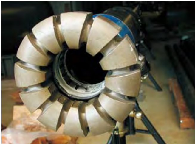
Figure 2. The core bit and core catcher assembly.
