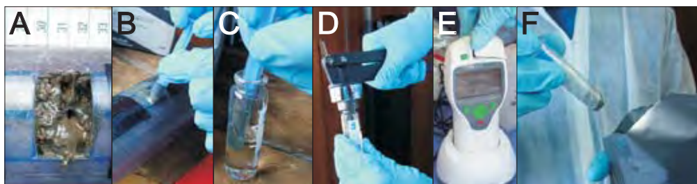
Figure 3. [A] Window cut for sampling; [B-D] sampling for methane headspace determinations; [E] preparation of the sample for in situ ATP measurements: sample is mixed with deionized water prior to centrifugation, then tested with the Uni-Lite ® NG water tester (shown); and [F] storage of the remaining sediment for cell culture. Refer to text for details.
