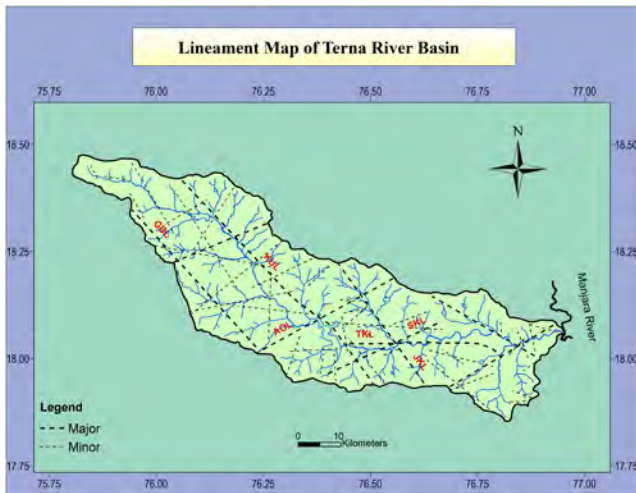
Fig. 3: Lineament map of the study area showing lineaments occurring along NE-SW, NW-SE, E-W and WNW-ESE directions (Modified after ARYA et al. 1995 and SRIVASTAVA et al. 1997). TKL – Terna-Killari Lineament, SKL – Sastur-Killari Lineament, AOL – Ausa-Osmanabad Lineament, JKL – Jawalgalana-Killari Lineament, KUL – Kallam-Umarga Lineament, GBL – Ghod-Bhima Lineament.
