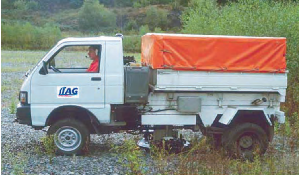
Fig. 8: Seismic hydraulic vibrator, constructed for near surface high resolution profiling.
