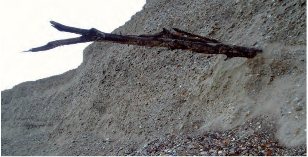
Fig. 2: Picture showing the position of the samples under study. A trunk is intercalated in sandy sediments (sand lense). The trunk was sampled for radiocarbon dating. Two samples were taken from sand about 20 cm below (LUM1220) and about 20 cm above (LUM1219) the trunk.
