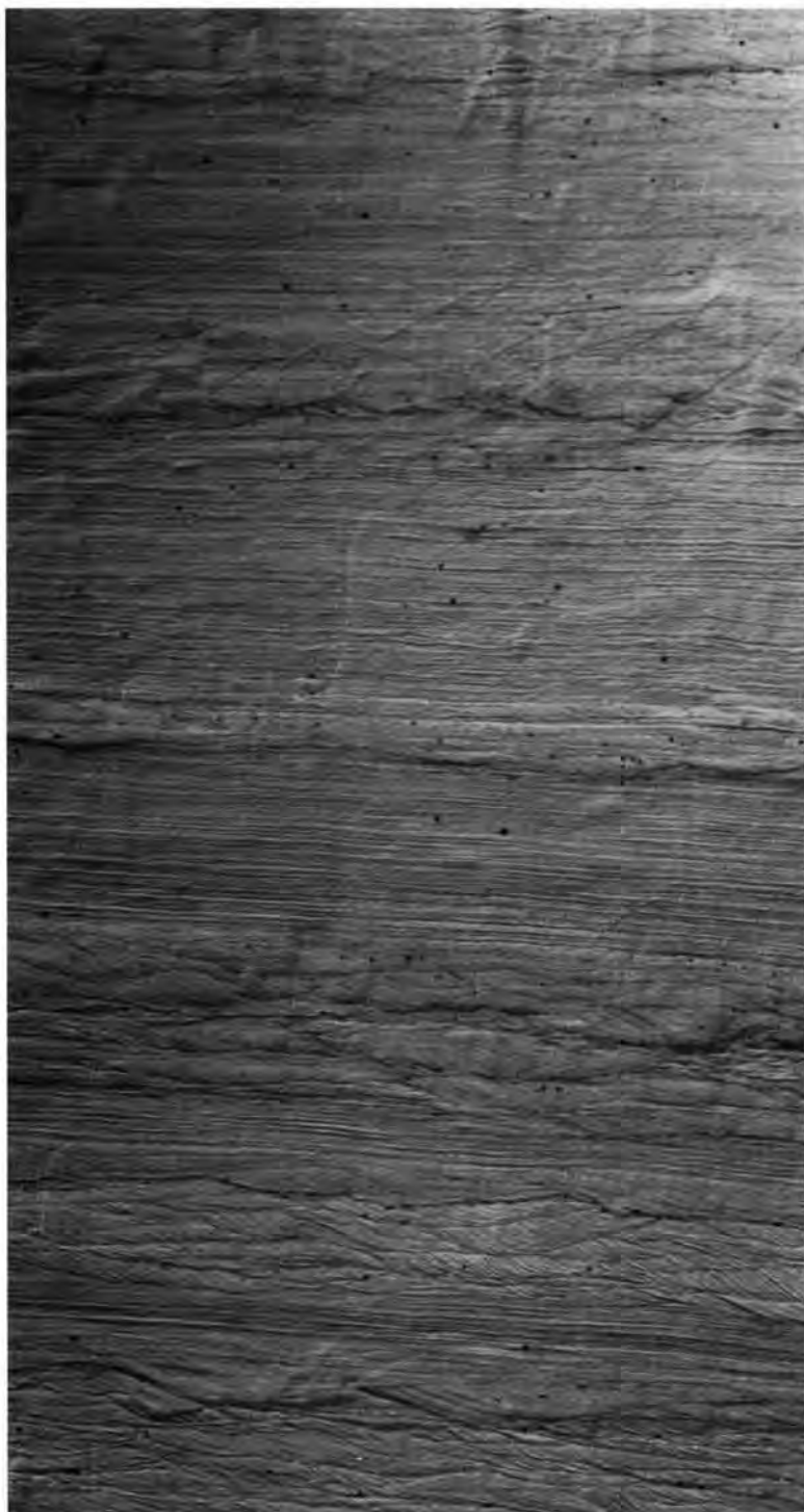
Fig. 10: Alternation of planebedded and ripple-laminated sets in incomplete turbidites of glaciolacustrine facies A. Scattered black mottles are lignite fragments. Lacquer peel from exposure Wattberg. Length of profile = 125 cm.
