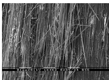
Fig. 1. BSE image of anthophyllite-asbestos.
