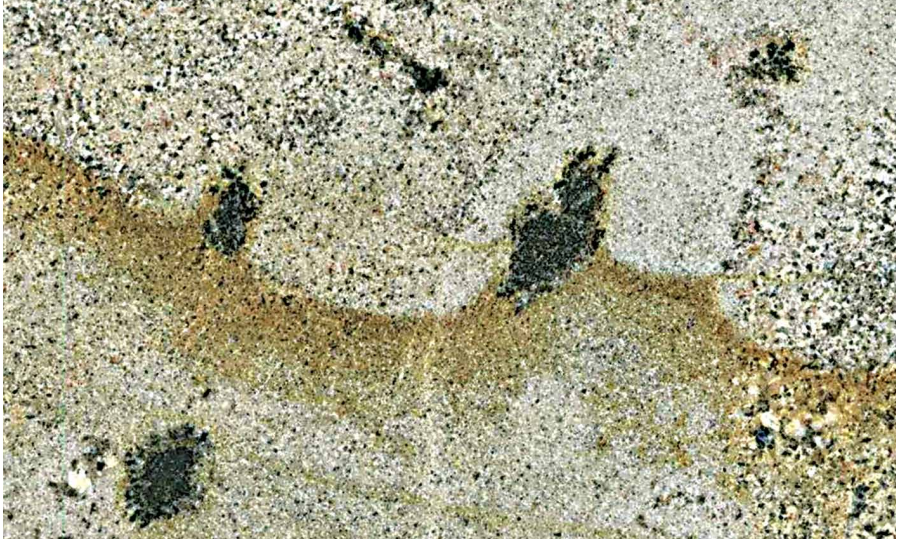
Figure 6.7.1. Polished slab of the leucocratic biotite aplogranite with dark brown clusters of sekaninaite (actual size). Photo J. Klomínský.
