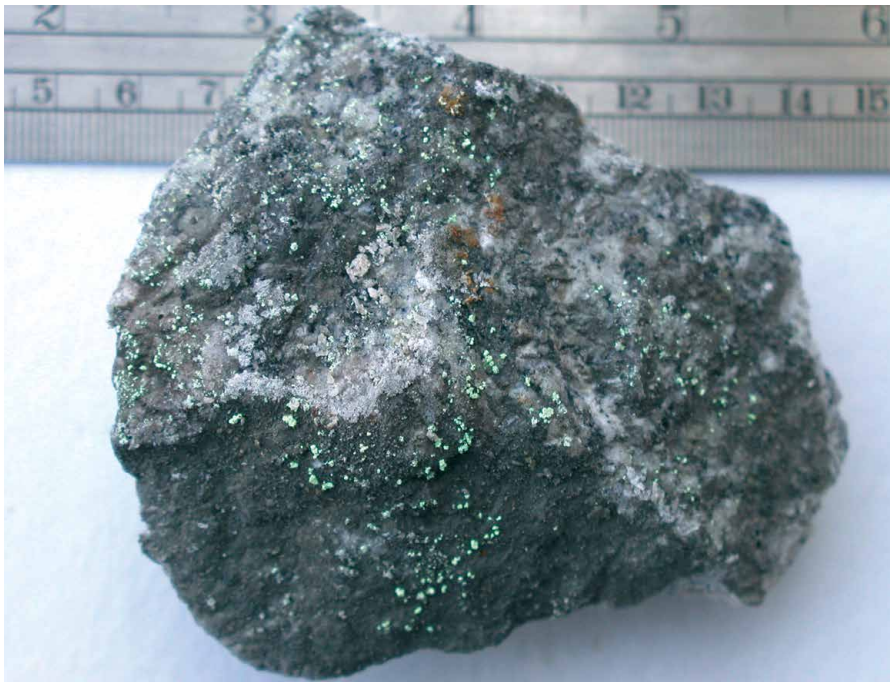
Figure 6.9.4. Schrockingerite crystals (yellow-green) and coatings of uranium-bearing opal (white) on the surface of Jizera Granite in the blasted excavation section of the Bedřichov water-supply tunnel section A. Klomínský et al. 2013.
