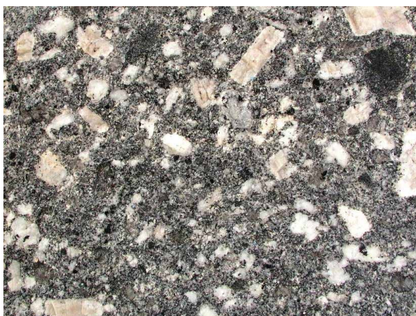
Figure 3.1.8. Žulový Vrch type hybrid granodiorite from the abandoned quarry in Rudolfovo (1/2 size). Photo J. Klomínský.
