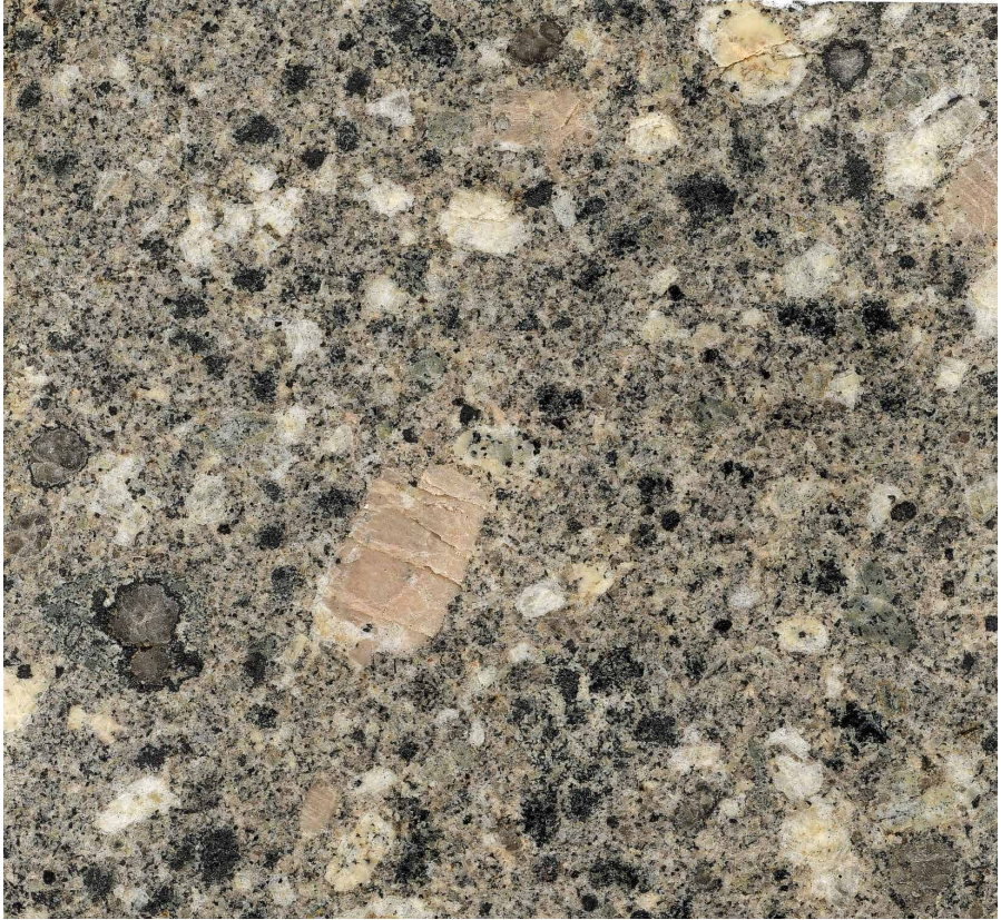
Figure 3.1.9. Novina type hybrid granite from outcrops near Novina village (real size). Photo J. Klomínský.
