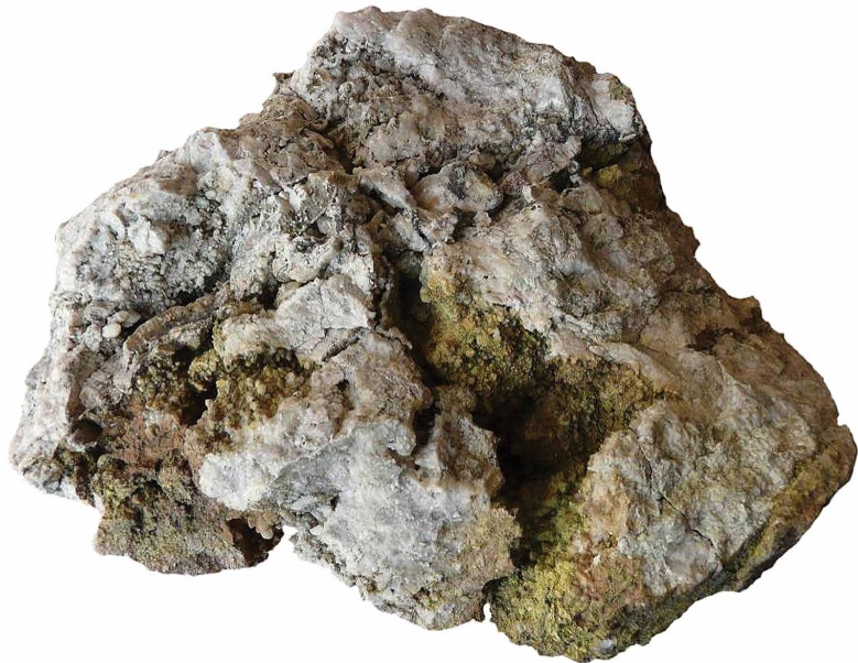
Figure 4.5.5. Fragment Vratislavice fault zone quartz vein with frequent open caverns (half of actual size). Photo J. Kломínský.
