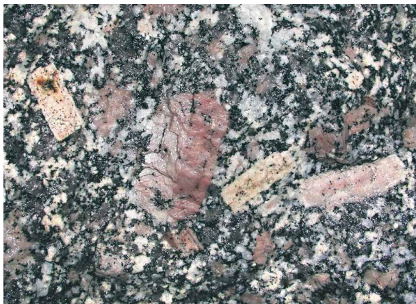
Figure 3.1.3. Different generations of K-feldspar phenocrysts in the Jizera Granite in the Souš water-supply tunnel. Size of the pink phenocryst is 5 cm. Photo J. Klomínský.
