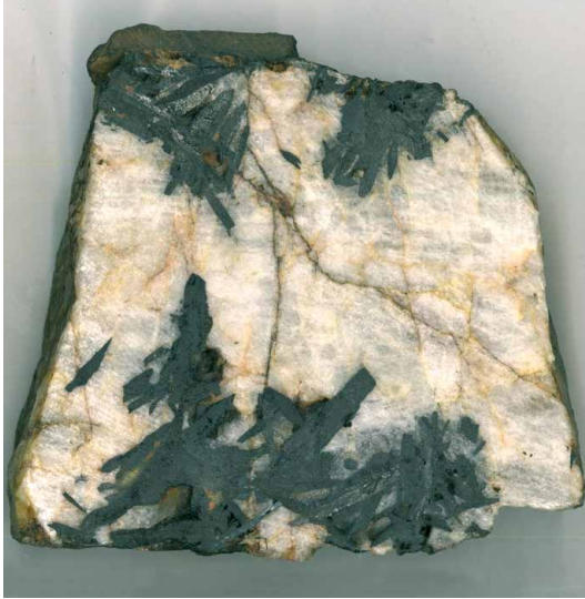
Figure 6.3.3. Clusters of wolframite crystals in quartz vein (natural size). Photo J. Klomínský.
