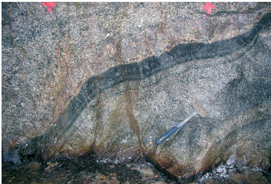
Figure 3.7.2. Folded composite multiple biotite schlieren in the Jizera Granite. The Souš water- supply tunnel. Photo J. Klomínský.
