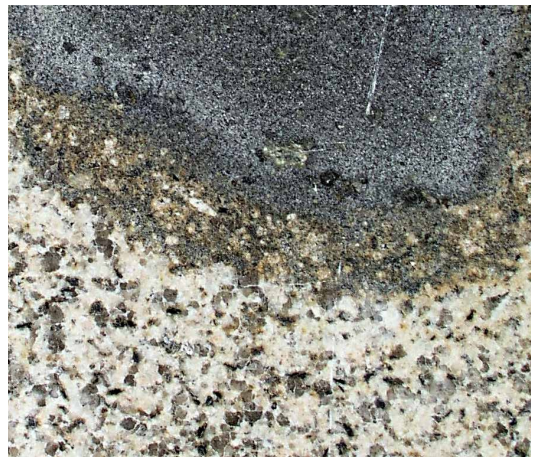
> Figure 3.7.13. Xenolith of quartzite with amphibolite in the Jizera Granite, Bedřichov water-supply tunnel section A (real size). Photo J. Klomínský.
