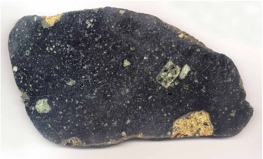
Figure 3.9.4. Tertiary olivine basanite with olivine xenocrysts and Tanvald Granite xenolith. Photo J. Klomínský. Exocontact of Tanvald Granite Massif in Hut' village near Jablonec nad Nisou (1/2 of the original size).
