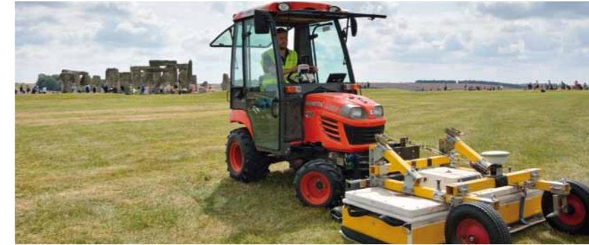
Bodenradaruntersuchung in Stonehenge Ground-penetrating radar investigations in Stonehenge
