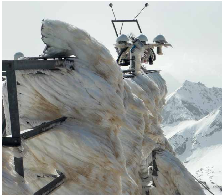
Saharastaub am Raureif der Messplattform Saharan dust over the hoarfrost on the measuring platform
