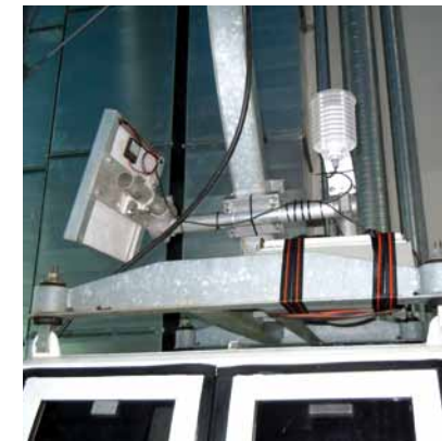
Mess-Sensoren am Dach einer Gondel Measuring sensors on the roof of a gondola
