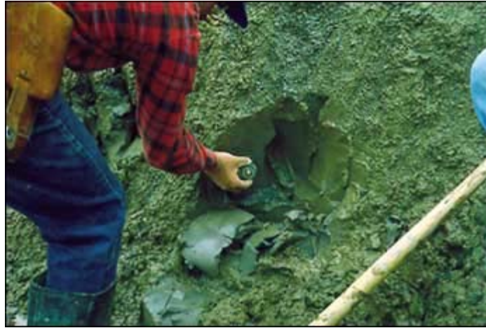
Figure 4. USGS and Syracuse University scientists using a vane shear device to measure undrained shear strength of an exposed stratum of glacial lake clay at the top of the 1993 Tully Valley landslide.
