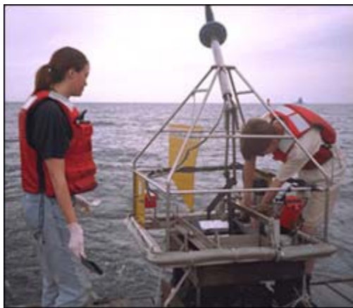
Figure 2. Photograph of the modified Van Veen grab sampler used to collect samples from the sediment surface, as well as to videotape and take still photographs of the sea floor.
