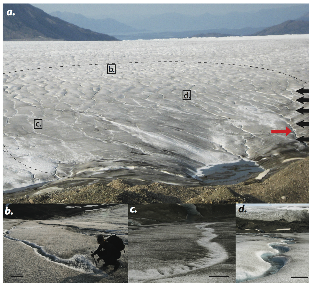
Fig. 2. (a) Marginal region of the Llewellyn Glacier that contains the study drainage basin (dashed line), photo taken from medial moraine. Black arrows indicate starting locations of survey transects, while red arrow is the stream in which the DTS temperature sensor was deployed. Boxed letters provide approximate locations of photographs in subsequent panels. (b) Inception of a supraglacial channel high in the upper study drainage basin, with porous icy substrate surrounding. (c) Recently abandoned channel, note difference in color between recently wetted channel ice and the glacier surface. (d) Example of a highly regular meandering reach. Black scale bars in panels (b–d) are approximately 50 cm.
