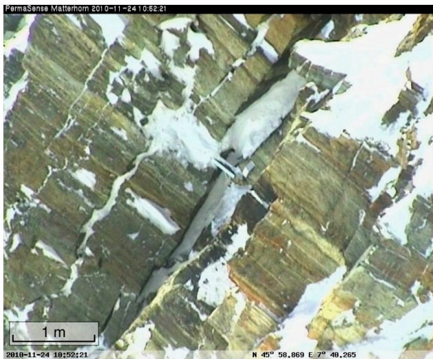
Fig. 5. Fractures with large spacing and aperture at Matterhorn Hörnligrat (pict. from November 2010).
