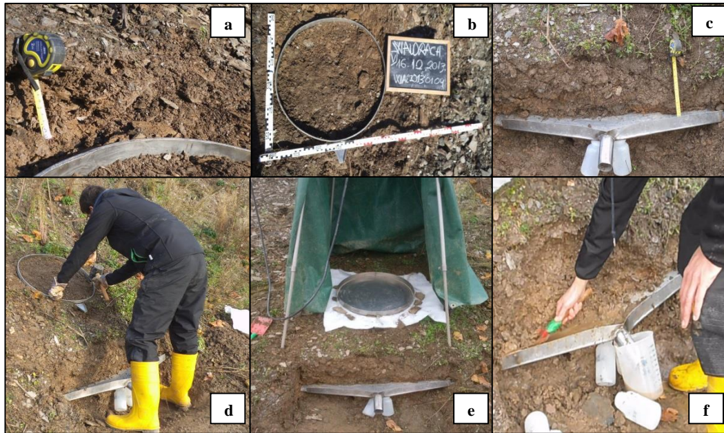
Figure 2. The rainfall simulation in December: (a) A horizon eliminated (between 5 and 7 cm); (b) before simulation; (c) profile to 0.5 m below ( 1.5 \text{ m} \times 0.5 \text{ m} ) with the sediment collector; (d) situation of simulator ring; (e) concurrent rainfall simulation, (f) subsurface flow during the experiment.
