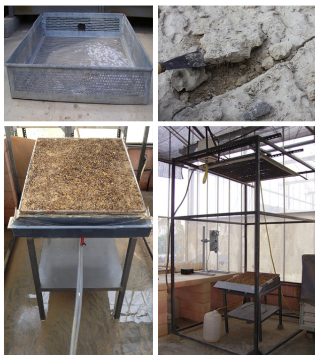
Figure 1. Experimental equipment and crust formation.
