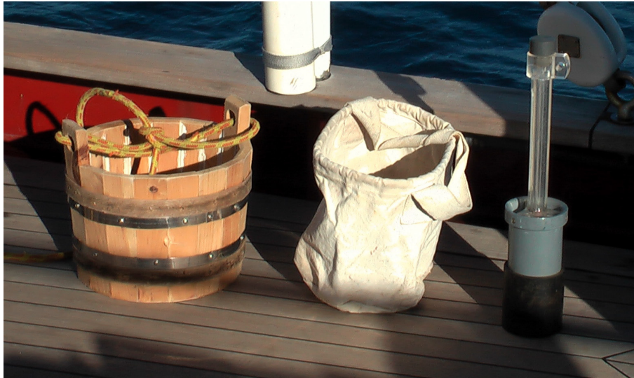
Fig. 2. From left to right, the wood, canvas and rubber buckets used in our field comparison. Note that the wooden bucket was sealed with white caulking along the inner seams and reinforced around the outside by two stainless steel bands. The rubber bucket is of both plastic and rubber construction, with a black rubber protective layer around the base.
