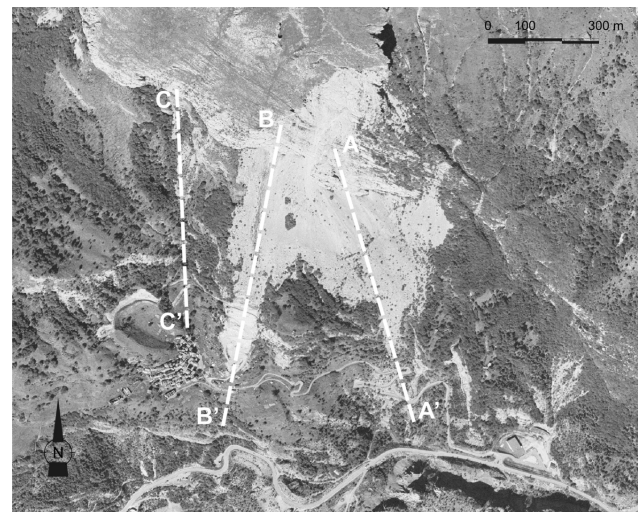
Fig. 3. The three numerically modelled cross sections of Monte Salta landslide slope.
