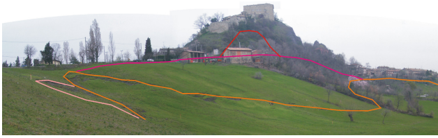
Fig. 1. Panoramic view of the higher part of the Rossena Landslide. Keys: orange line = main body (rotational), purple line = earth slide (translational), red line = rock slide, pink line = secondary landslide.
