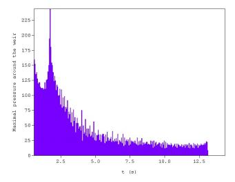
**Fig. 7.**  $P_{\text{max}}$  (Pa) versus time around the obstacle.
