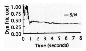
**Fig. 1.** Results of experiments (Dent et al., 1998) with snow:  $\frac{S}{N} = cste$ .
