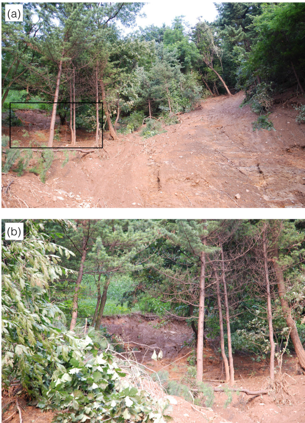
Figure 6. Landslides in Site C. (a) Landslide initiation zones, looking northeast. An area outlined by a black solid line presents a closer look of one of the initiation zones in slopes (b). (b) A closer look of the landslide initiation zone indicated in (a).
