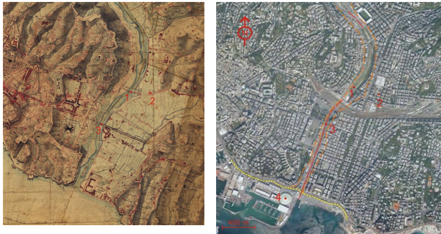
Figure 6. Final stretch of the Bisagno stream at the beginning of the 19th century (left panel) and in the present day (right panel). Note the complete urbanization, the progradation to the sea in Piazzale Kennedy area and Fiera del Mare (4) and the narrowing of the flow section near S. Agata bridge (1) and of Pila bridge (S. Zita) (3). Number 2 shows the Sant'Agata Cloister, where the left pier of the bridge rose (280 m length). Note that the stream has been completely culverted downstream from the railway since the 1930s (red dashed line). The orange dashed line indicates the Bisagno stream banks at the beginning of 1800; the yellow dashed line indicates the shoreline at the beginning of the 19th century.
