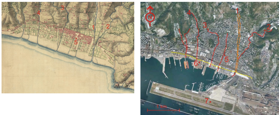
Figure 7. Comparison of the final stretch of the Chiaravagna stream 1821 and today. Note the urbanization of the plain, shipyards (6), the old small harbour and the airport (7) and the railway. It is possible to observe the strong progradation to the sea, the covering of the Chiaravagna stream (1), whose banks are indicated by a dashed orange line, and the Rio Ruscarolo creek (2), whose deviation has directed its flow into the Chiaravagna stream and not to the beach. Numbers 3 and 4 indicate the Molinassi and Cantarena Streams (dotted red), number 5 is the Church of N. S. dell'Assunta in the historic centre of Sestri Ponente. The dashed yellow line indicates the shoreline at the beginning of the 19th century.
