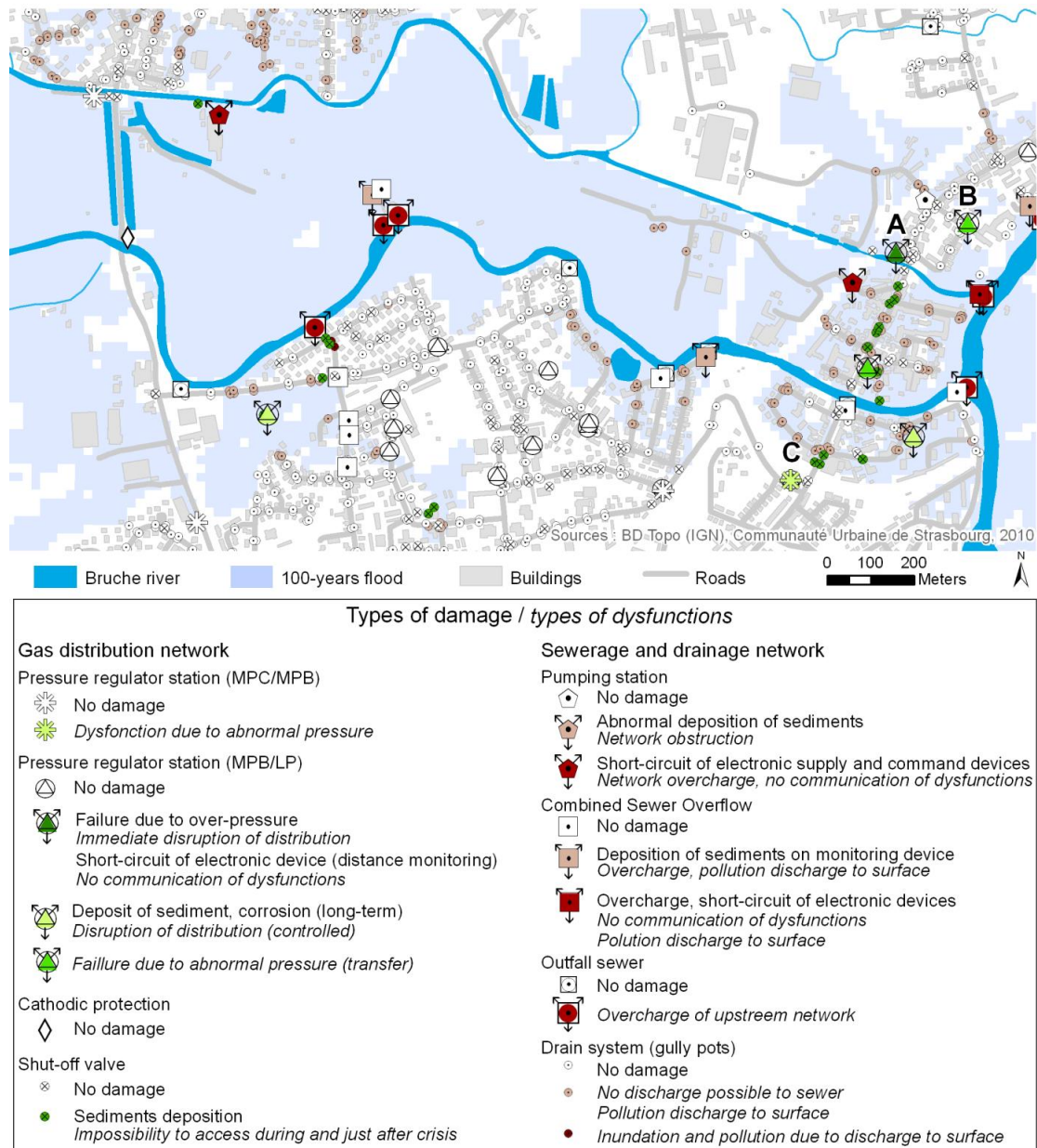
Fig. 6. Map of damage-dysfunctions caused by a 100-year return-period flood for the components of gas distribution and sewerage/drainage networks.
