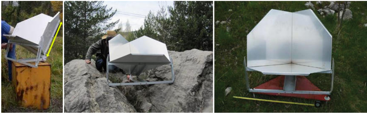
Fig. 2. Corner Reflectors (CRs) used to monitor the Vallcebre landslide. The yellow arrow indicates the size of the side of the CRs which is 67 cm. Three types of CR installation were performed in the Vallcebre landslide: over a metallic box, on rocks or directly over the terrain.
