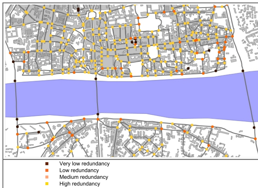
Fig. 6. Orleans road networks redundancy analysis shows the weak redundancy of this network close to bridges.
