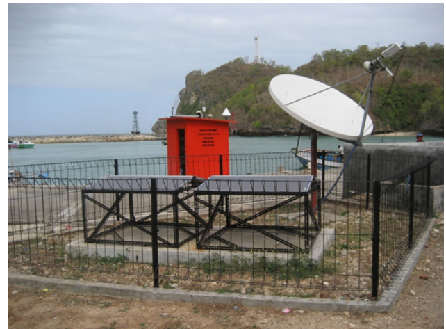
Fig. 2a. An example of a GPS-controlled tide gauge station (Sadeng, Java/Indonesia) of the GITEWS project in support of the InaTEWS system of Indonesia. The station is equipped with radar, float and pressure gauges. The GPS antenna is mounted on the top of the tide gauge hut. In addition, the meteorological sensor is visible as well as some antennas for data transmission.
