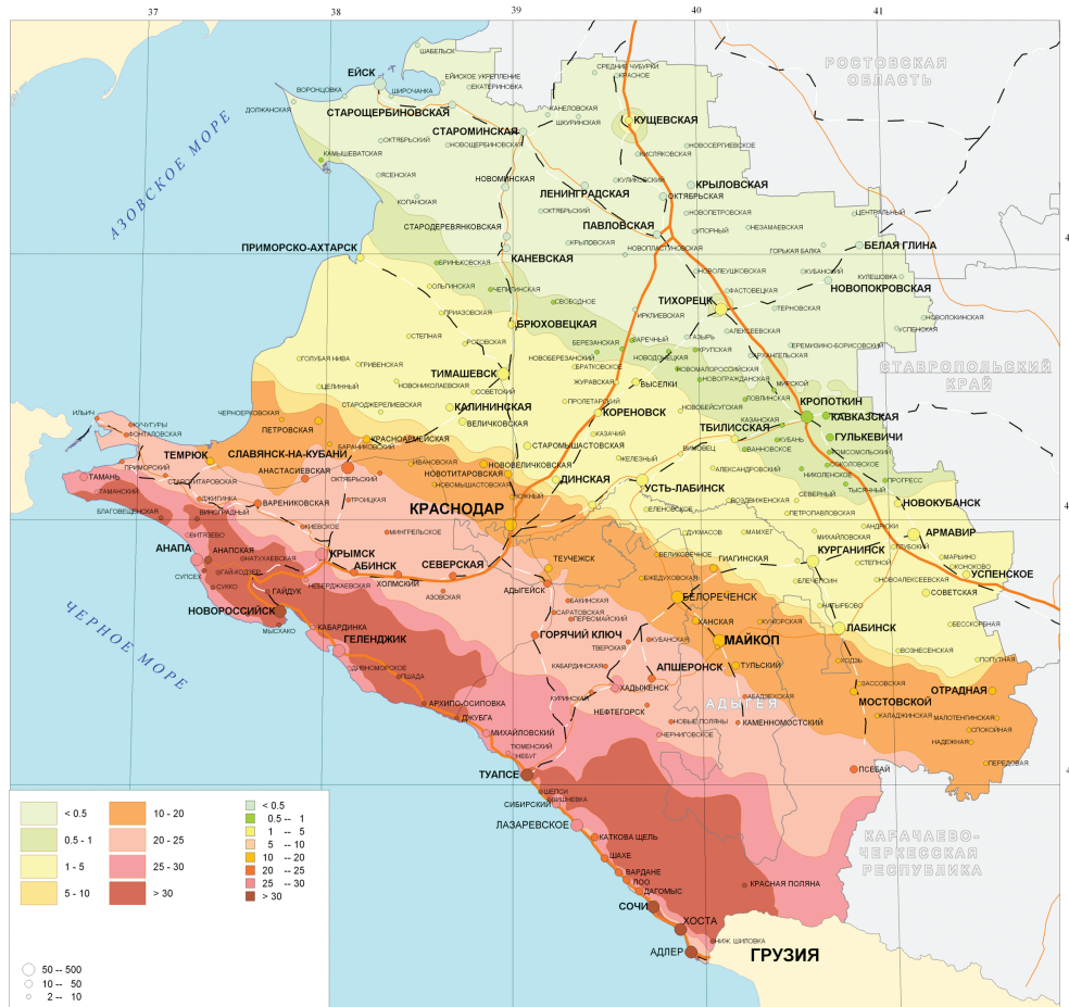
Fig. 2. Map of seismic risk R_{st1} , 10^{-5} \text{ yr}^{-1} zoning for the territory of the Krasnodar region, taking into account technological accidents triggered by earthquakes.
