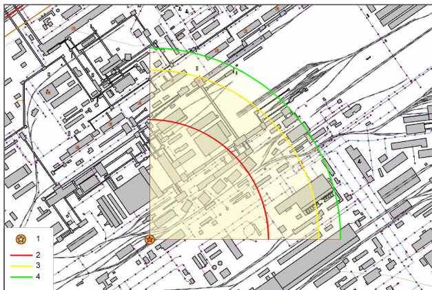
Fig. 6. Simulation of possible contaminated zones in the case of an accident with chemical material release: 1 – source of release of 3.0 tons liquid chlorine; 2 – after 1 h; 3 – after 3 h and 4 – after 4 h.
