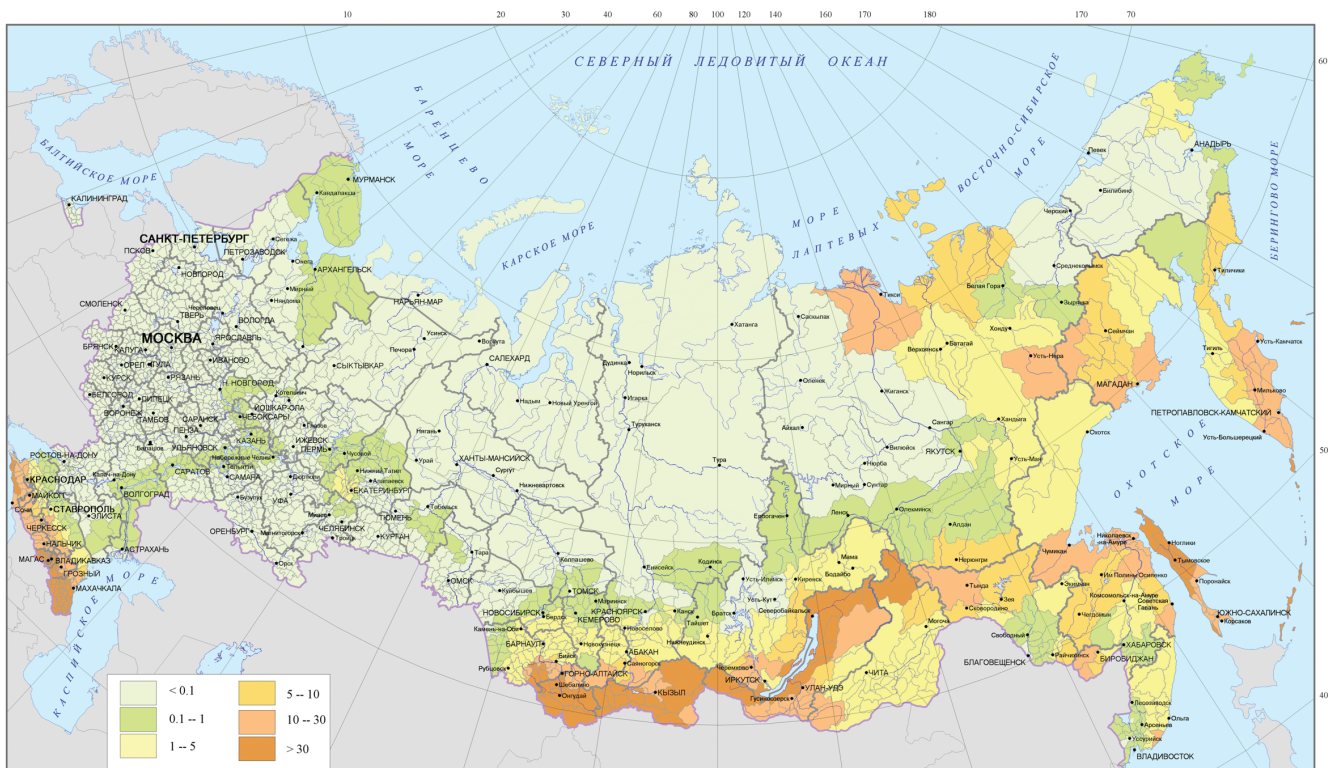
Fig. 1. Map of individual seismic risk R_s1 , 10^{-5} \text{ yr}^{-1} , for the territory of the Russian Federation.
