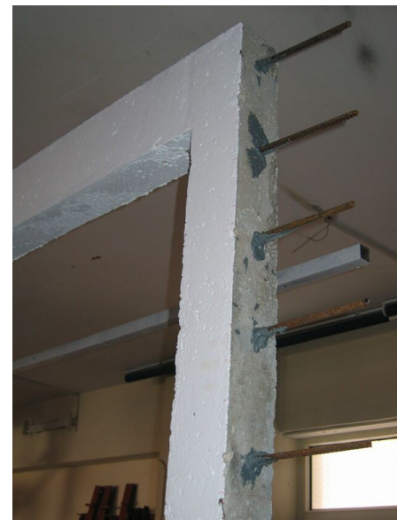
Fig. 2. Properties of anchor dowels (Arslan et al., 2010).
