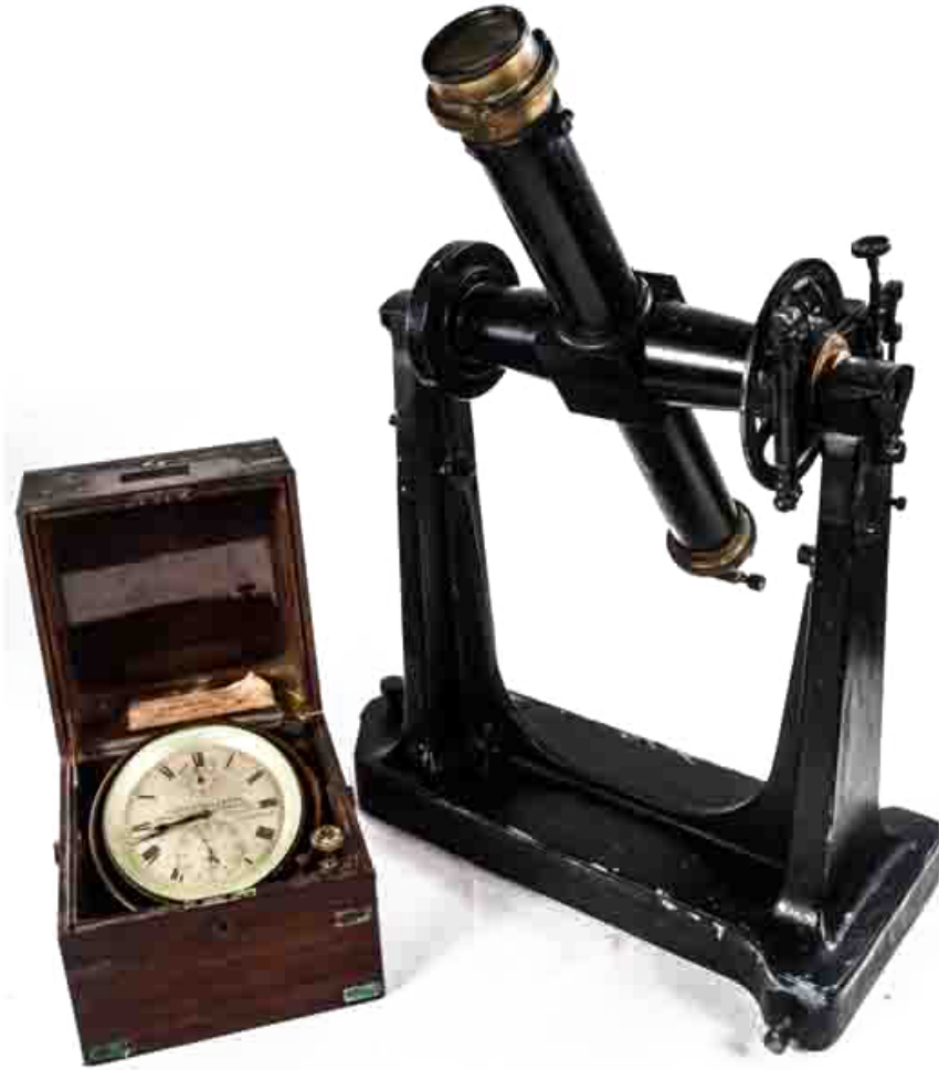
Figure 22. Transit telescope and chronometer (courtesy of Colaba–Alibag Observatory).
