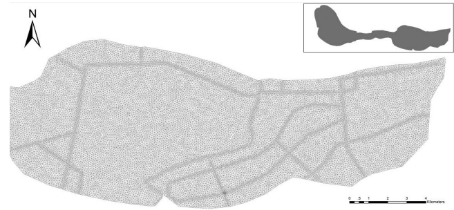
Figure 4. The two-dimensional (2-D) hydraulic model mesh of the Gongshuangcha detention basin and its regional enlarged view.
