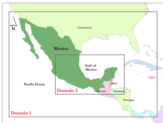
Figure 2. Numerical setup of the WRF with a nested domain covering Mexico. Domain 1: 25 km resolution; Domain 2: 4 km resolution; the orange region illustrates the Tonalá catchment.
