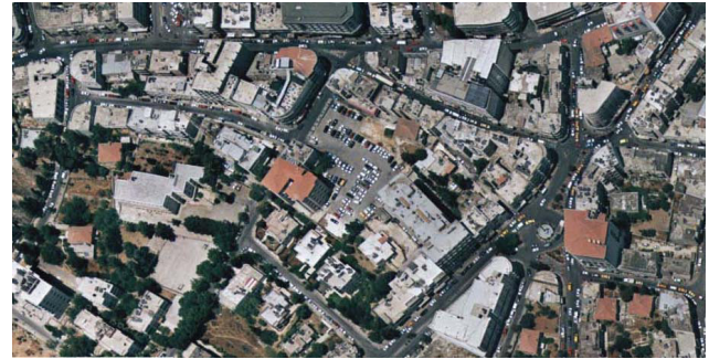
Fig. 9. Detail of the orthophoto used for GIS-analysis: the two dominant roof types in Ramallah can be identified: flat concrete roofs (grey) and sloping clay tile roofs (red).
