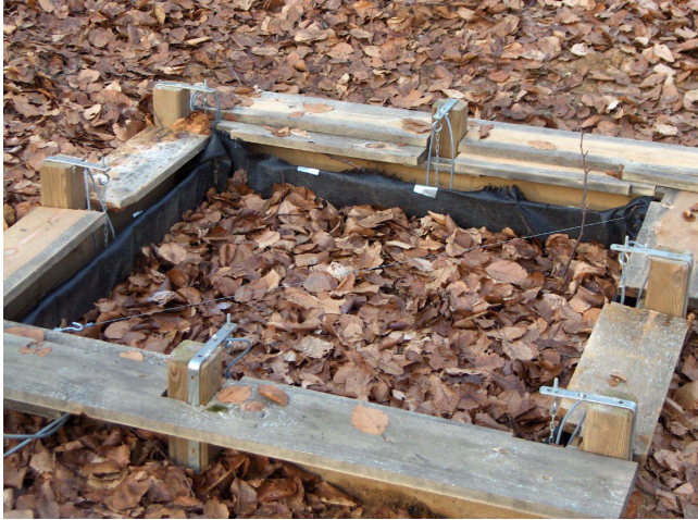
Fig. 3. Interception device in the Huewelerbach catchment on January 2006. The upper basin is filled with leaf litter.
