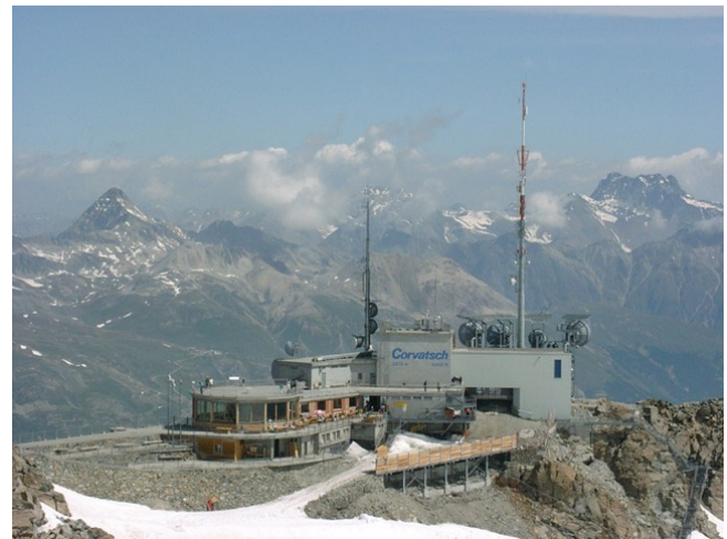
Fig. 3. The height of the meteorological station at Piz Corvatsch is assumed uncertain, ranging from 0.5 to 16 m. Within mountain topography, the actual height in relation with the surroundings at the top of a mountain cannot be accurately determined. In the figure, the meteorological station is just above the “tsch” of “Corvatsch”.
