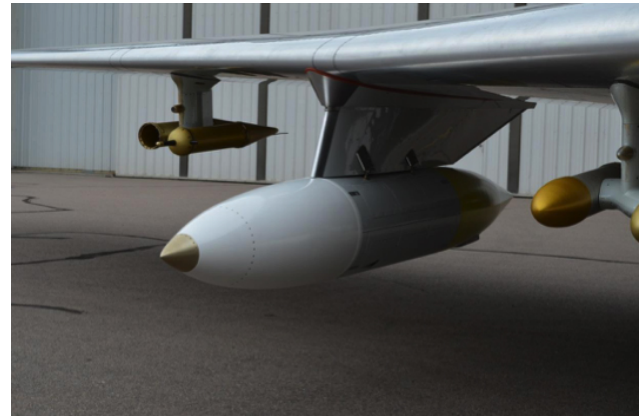
Figure 1. View of an NCAR pod mounted below the surface of the right wing.
