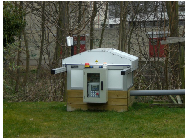
Fig. 4. Roll-off roof in real-sky test environment.
